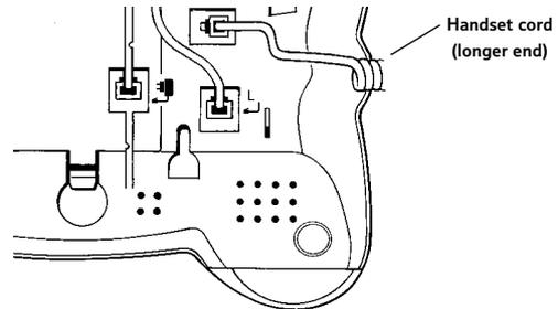
2. Connect the telephone line cord and mains power cables to the underside of phone.
