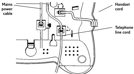
The base station must be plugged into the mains at all times.
