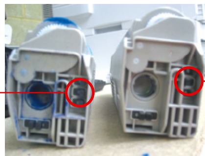
Q Imaging centre post in incorrect position (Source – OKI Printing Solutions)
