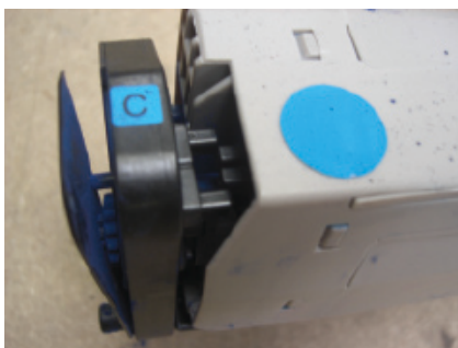
Q Imaging Cyan image drum forced open after 1,000 pages through incorrect positioning of centre post (Source – OKI Printing Solutions)
